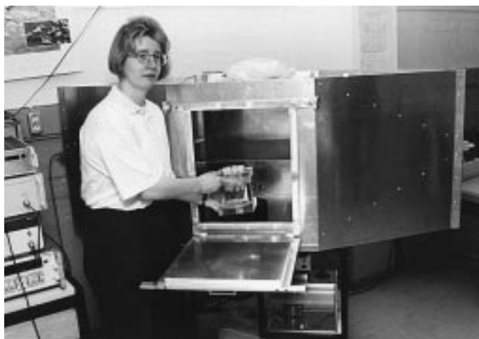
Introduction of the test tube into the GTEM cell; on the left: equipment to generate and measure the high frequency electromagnetic fields; the permanent control and data recording of the field strengths is safeguarded by a computer control device.
