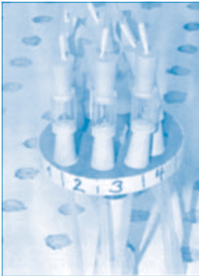
Figure 18: Test chambers designed for direct exposure of pineal organs to weak magnetic fields. In each chamber pineal organs of adult Djungarian hamsters were perfused with buffer solution. Subsequently, in the eluate melatonin was determined. For melatonin production it is necessary to pharmaceutically stimulate the organs. Taken from [137].
