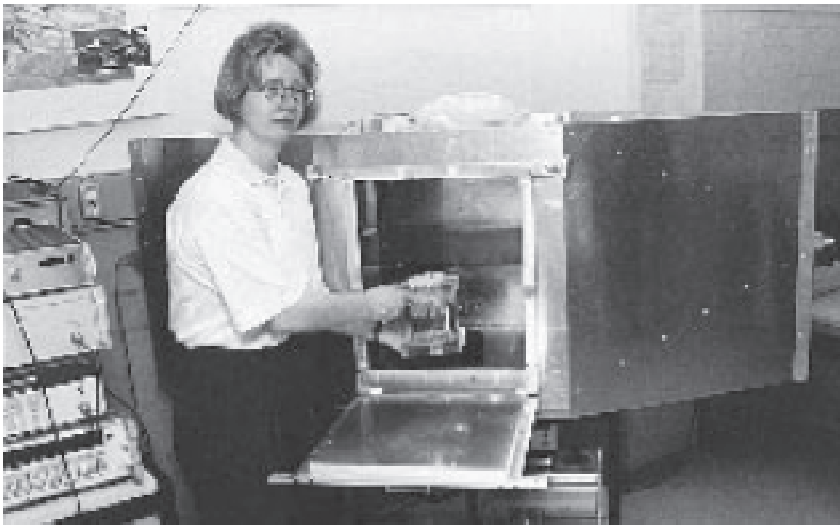
Insertion of the sample holder, with samples, into the TEM cell. On the left side of the picture, equipment for the generation and measurement of radio-frequency electromagnetic fields is depicted. Both the measurement procedure and the recording of the field-strength values are carried out under computer control.
