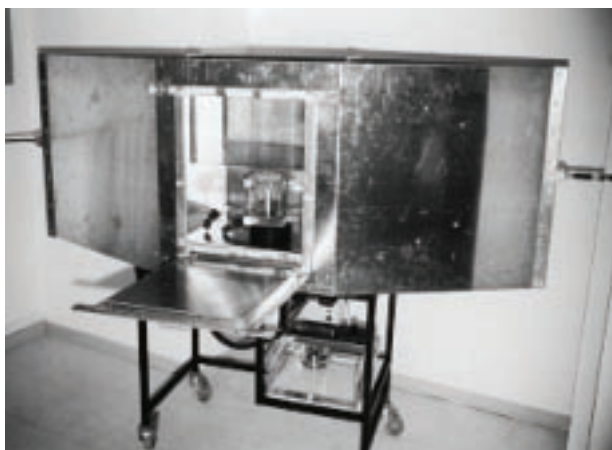
Fig. 6: TEM cell used in the experiment, with one side wall opened to permit a view into the cell interior. In the lower part of the cell interior, the sample holder with nine culture containers can be seen. Above this is the isolated suspended septum, which is the extension of the inner conductor of the coaxial feed line, present on the figure's right-hand side. The thermostatically-controlled bath is located outside the TEM cell.
