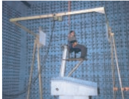
Figure 4: Experimental set-up in low-reflection room
