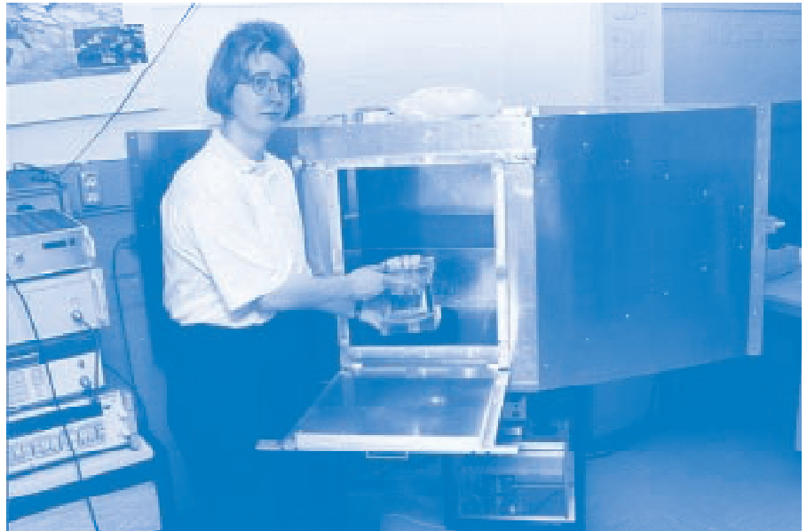
Fig. 4: Inserted TEM cell (450 MHz) in biological in vitro experiments (TU Braunschweig)
