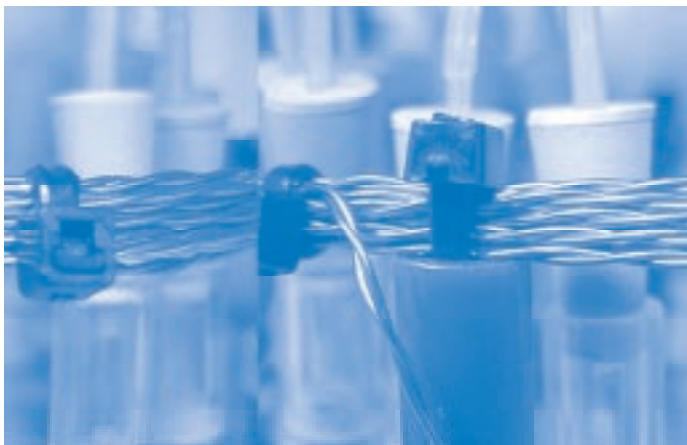
Fig. 5: Test chambers designed for direct exposure of pineal glands to weak magnetic fields. In each chamber pineal glands of Djungarian hamsters are flushed with a buffer (perifusion). Then, in the eluate, melatonin is determined. To produce melatonin, pharmacological stimulation of the glands is required. Taken from [100].
