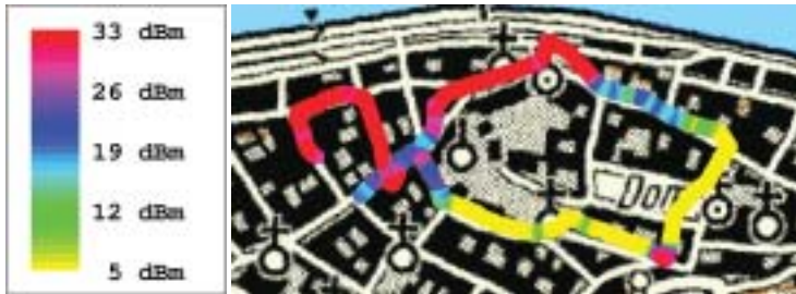
Fig. 5: Local distribution of transmission power along the measurement route 1 in Passau (measurement 1a)
