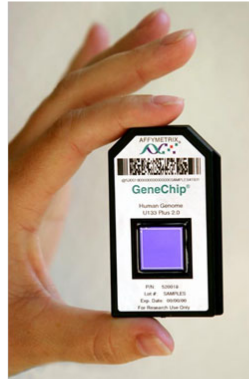
Affymetrix GeneChip® (up to 1.3 \times 10^6 25mer oligonucleo- tides, in situ synthesis)
