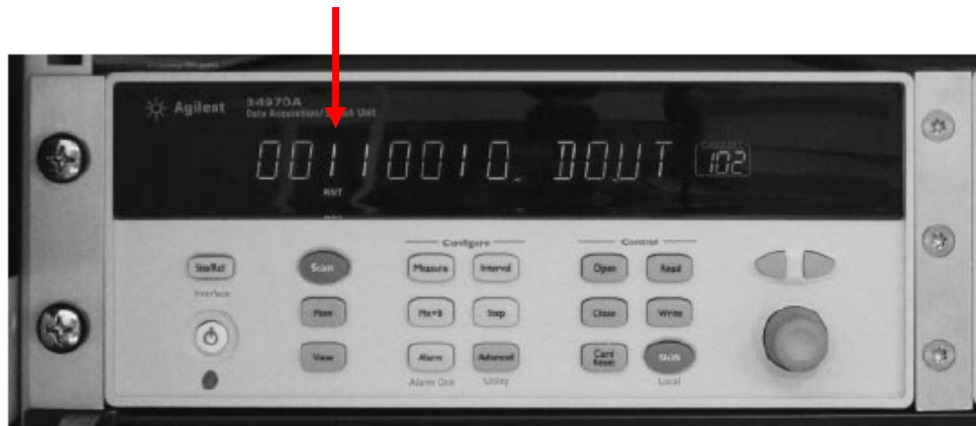
Fig. 1. Display panel on the Agilent 34970A Data Acquisition/Switch Unit: switched to channel 102. Third digit in eight-digit number (left) indicates waveguide in use (0 = waveguide 1, 1 = waveguide 2).
